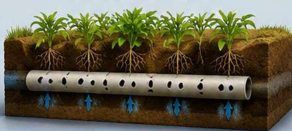
a) Subsurface Pipe Irrigation
